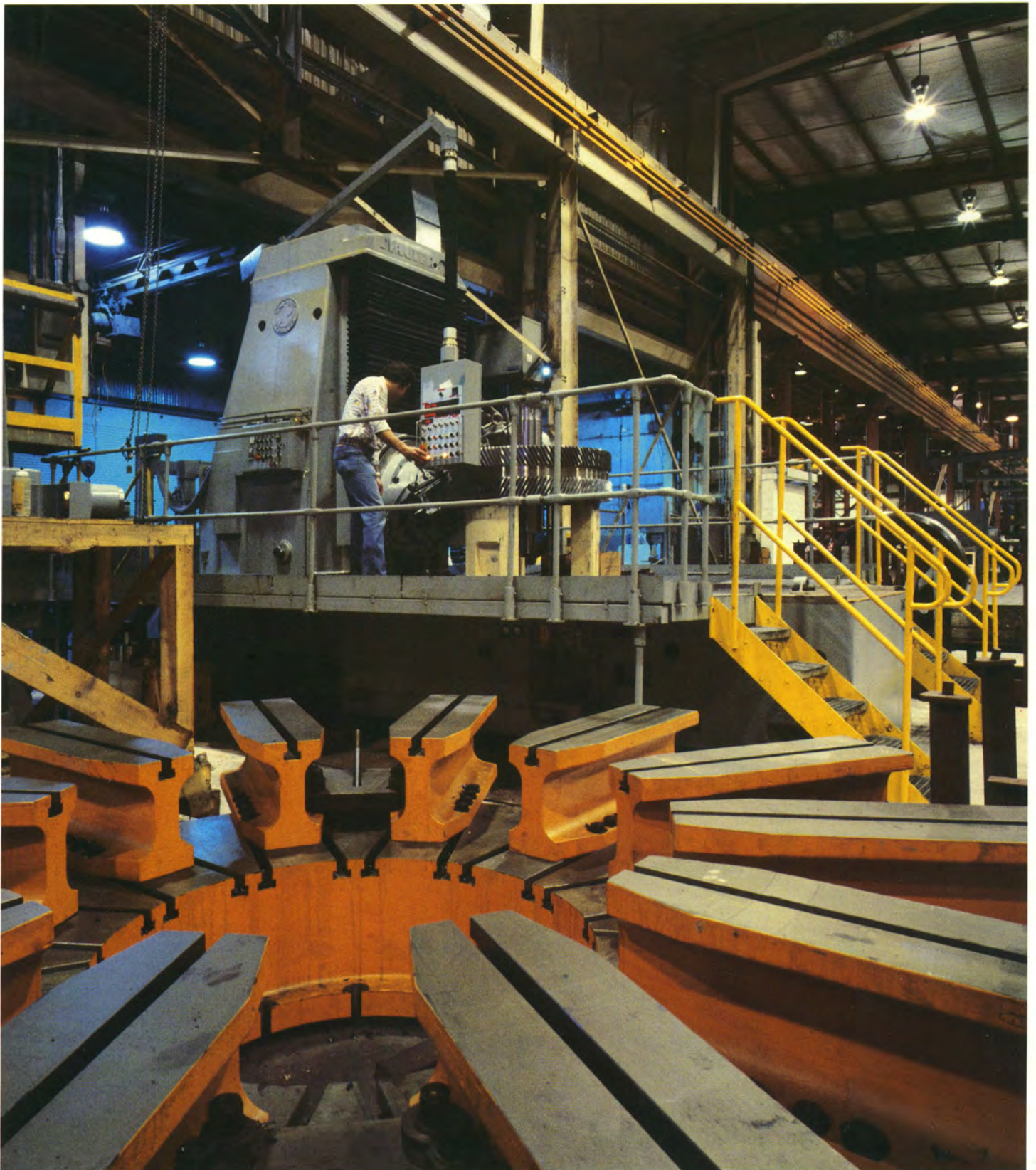
This special accuracy 120-inch gear hobbing machine features high speed roughing with a carbide gashing tool and precision finish hobbing.
