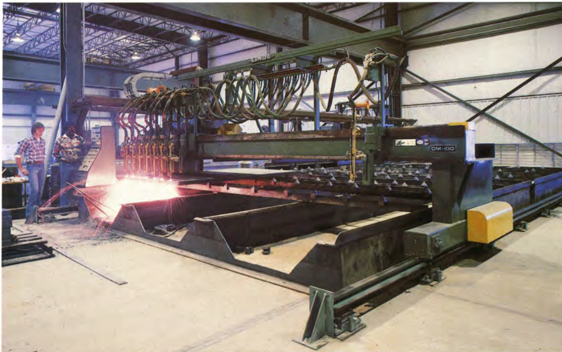
The new structural steel fabrication plant houses the optimum in welding equipment, including a computer actuated plasma arc shape burning machine (left) and a state-of-the-art torch cutting machine (below).
