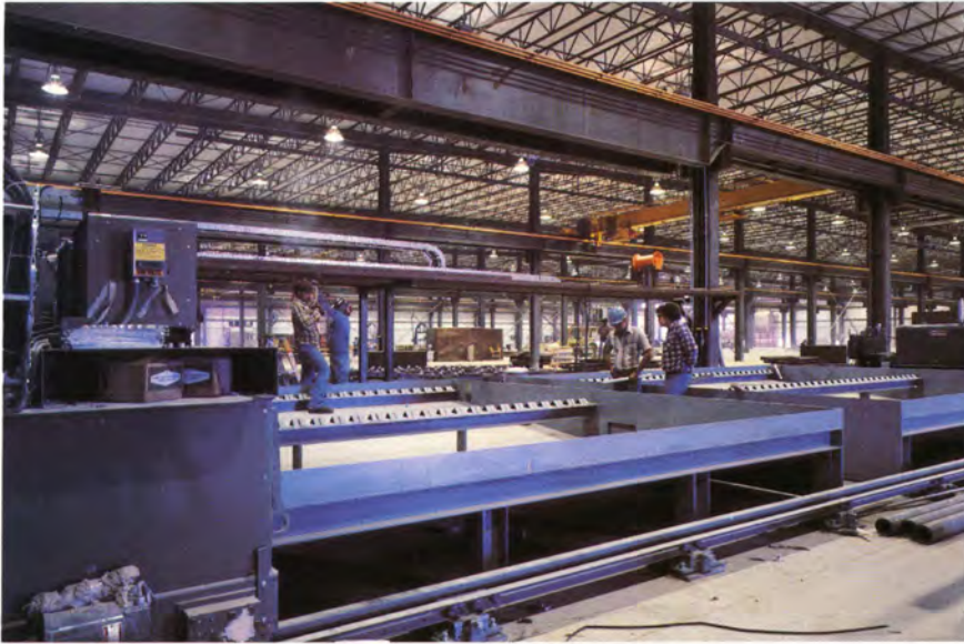
The new structural steel fabrication plant houses the optimum in welding equipment, including a computer actuated plasma arc shape burning machine (left) and a state-of-the-art torch cutting machine (below).
