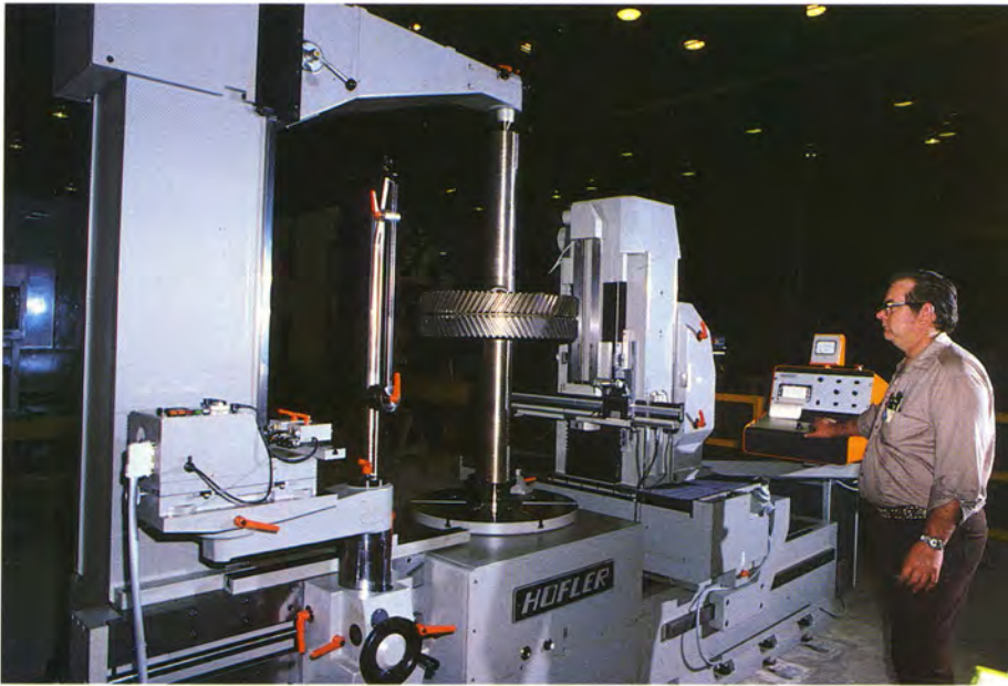
This gear-tooth checker, a capital investment in 1981, is an extremely precise machine used for industrial and marine gear quality assurance.
