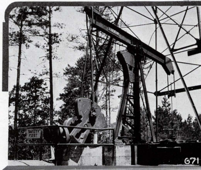
Photograph No. 671:—Loring Oil Company, Zwolle, La., Bowman-Hicks No. 6. Lufkin Baby Unit—Baby Crank, 15 H.P., 1200 R.P.M. FTR G.E. Motor, No. 2 Sampson Post assembly. Well 2450 feet deep, 3½-inch tubing, ⅜-inch rods, production 250 barrels per day, 42 gravity oil.
