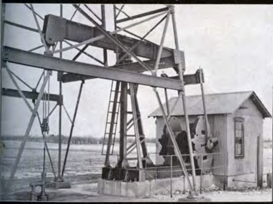
Lufkin TC-2-26 Unit, Lorraine, Kansas. This photo not retouched—being entirely covered with ice gives retouching appearance.
