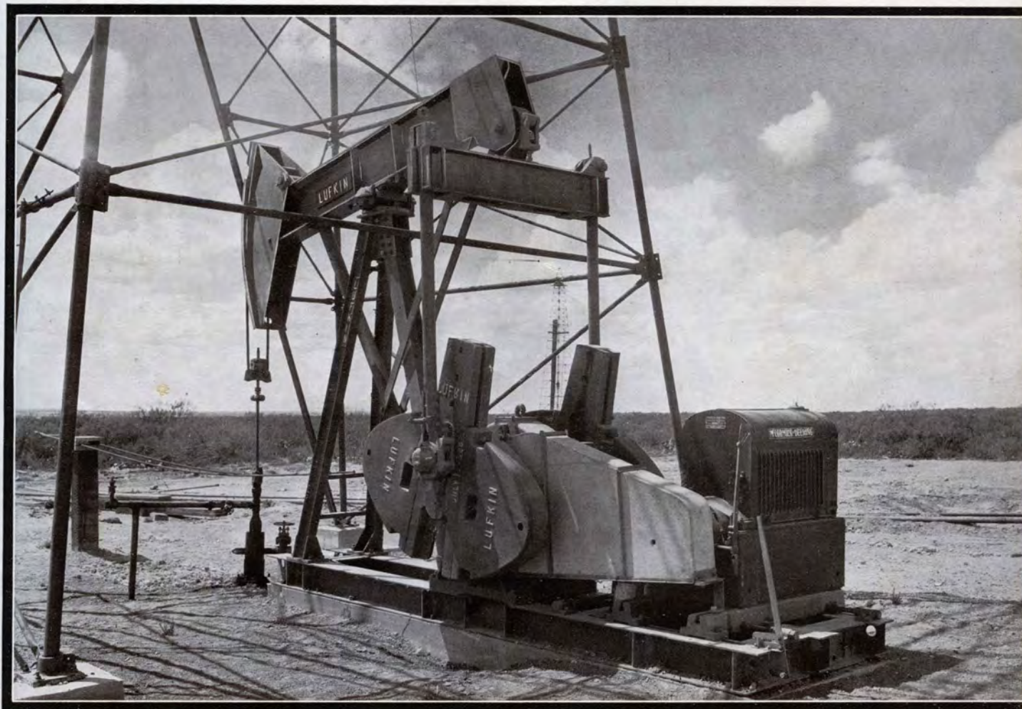
Magnolia Petroleum Company, Loma Novia pool, Government Wells field, Duval County, LUFKIN Unit Assembly T.C. No. 3-18 with gas engine drive.
