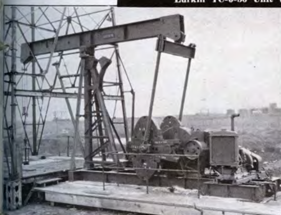
Lufkin TC-1A-58-1028-C Unit with 130-lb. Beam. Hercules engine. I. T. I. O. Corp., South Glendale No. 2, Oklahoma City.
