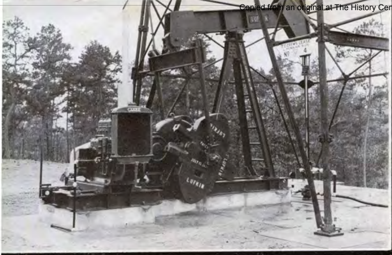
Continental Oil Company, C. C. Crews No. 4, L. Perkins Survey, Gregg County, East Texas — LUFKIN Unit Assembly T.C. No. 3-18, with Clark multi-cylinder gas engine drive.
