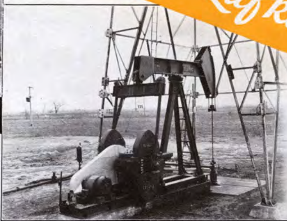
T. C. Johnson Oil Co., Wichita, Kansas. Lufkin TC-3-22 Unit with G. E. enclosed motor.
