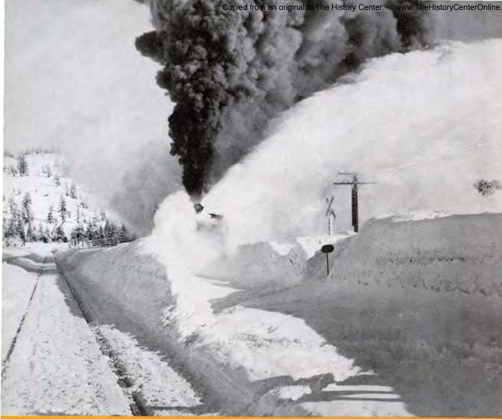
Left —Snow and plenty of it—Close up of a railroad rotary plow in action.
