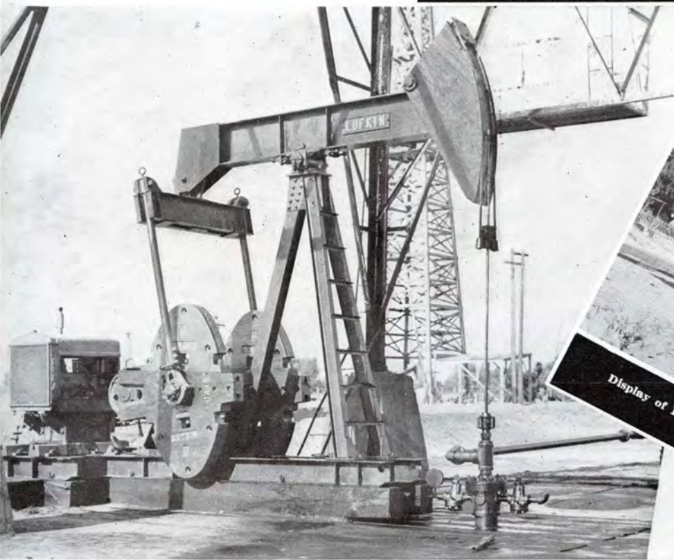
Western Gulf Oil Company, Fruitvale field, Lufkin T.C. 3-22 unit assembly.
