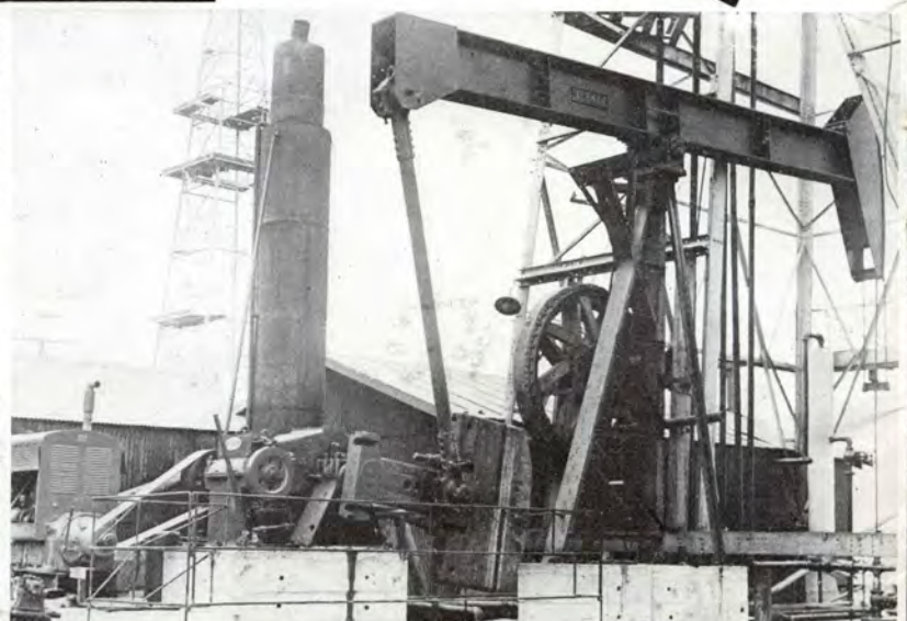
McVicar and Rood, Huntington Beach, California. Lufkin Unit S.C. 41 (Special 88-inch Stroke set up).
