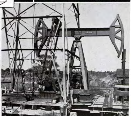
Lufkin Long Stroke Unit (120" maximum) No. 10-41, Magnolia Petroleum Company, Westlake, Louisiana. Note compactness.
