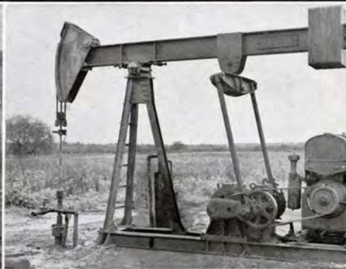
Lufkin T.C. 5-7 Unit with plain cranks and counterbalance, Luling Oil & Gas Company, Caesar Pool, Bee County.
