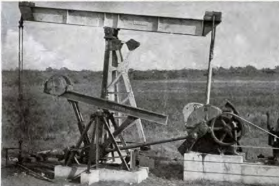
Luling Oil & Gas Company, Caesar Pool, Bee County. Lufkin No. 58 Unit with back side crank and counterbalance vertical swing.
