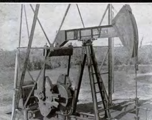
Pettus Refining Company, McKinney lease in the North Pettus field, Lufkin T.C. 3-18.
