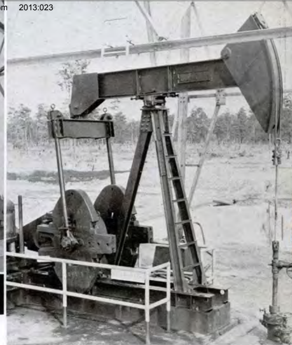
Houston Oil & Republic Production Company— Ariola X Fee No. 3, Ariola, Texas, Lufkin T.C. 2-31-B Unit.
