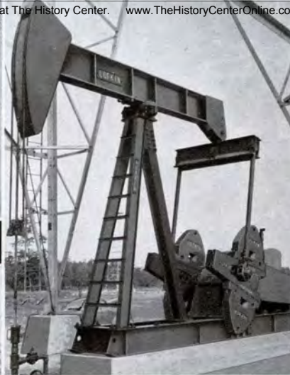
No. 1409 Lufkin T.C. 2-31-B Unit, Ariola X Fee—Republic Production & Houston Oil Company, Ariola Texas.
