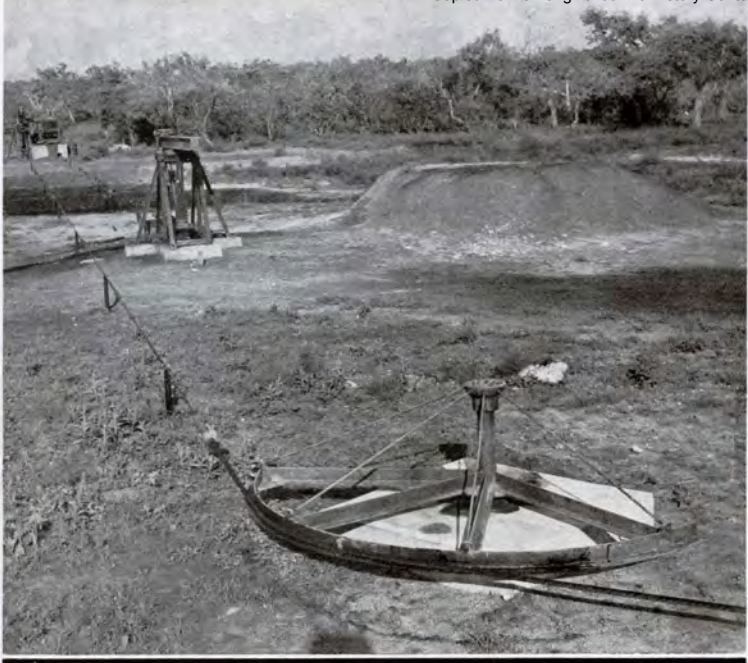
Lufkin Wire line swing, Major Oil Company installation in Bee County. NOTE Lufkin "Bull-dog" Unit in background, Lufkin Jack in center.
