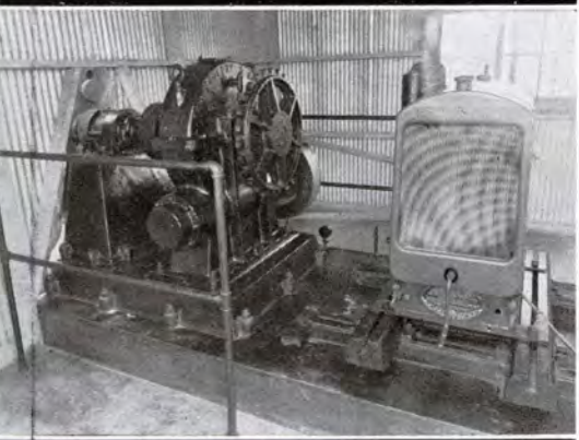
One of the early Lufkin units, built in 1925 and still in first class operating condition pulling two wells for a major oil company in Duval County. This is the old style worm gear unit with pedestal bearing, Unit No. 47.
