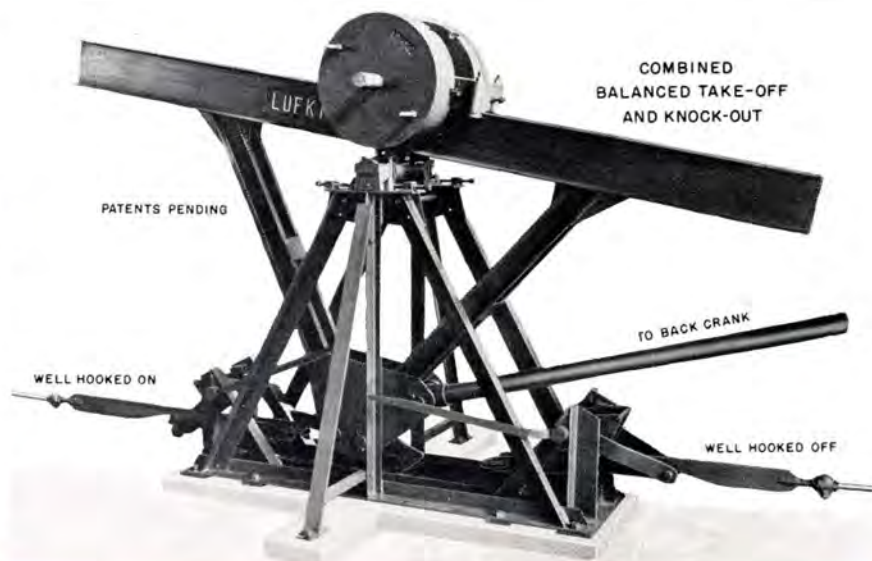
The Lufkin Combination counterbalance take off and knockout.
