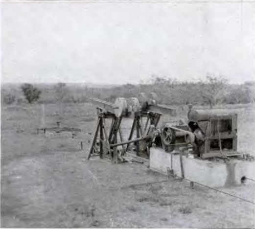
Lufkin No. 31 Unit with Lufkin counterbalance vertical swing pulling 4 wells, Luling Oil & Gas Company, Caesar Pool, Bee County.
