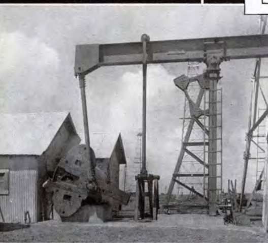
Woodley Petroleum Co., Blue Ridge, Texas. Lufkin S.C. No. 56 Unit with bell crank take-off for pumping additional wells.
