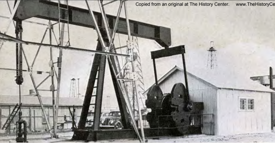
Typical Lufkin installation in the Talco, Texas, field. Magnolia Petroleum Co., W. H. Crawford No. 1, Lufkin T.C.-58 Unit with long base.
