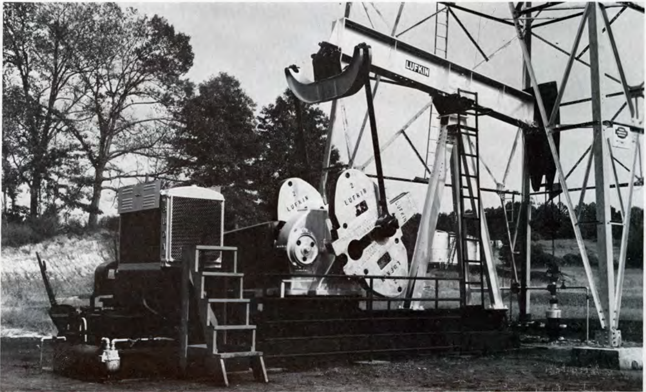
DISCOVERY WELL, Union Producing Co., Woodruff No. 1, the discovery well in the Tinsley, Mississippi, field—LUFKIN EQUIPT. Photo shows Lufkin Unit assembly T. C. 2A-36
