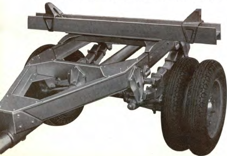
Lower left: The new all-steel, riveted and welded pipe and pole trailer, designed for long lasting service and continuous operation on the tougher jobs where ability to "take it" is a prerequisite.
