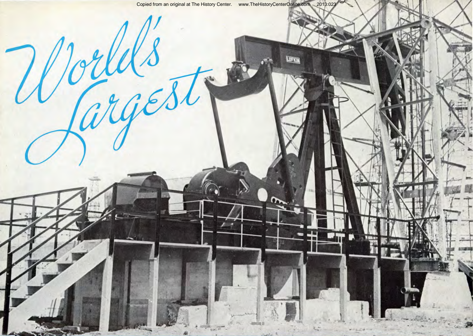
SEAL BEACH installation. Lufkin No. 71 Unit assembly having 750,000 in. lbs. torque gear rating.
