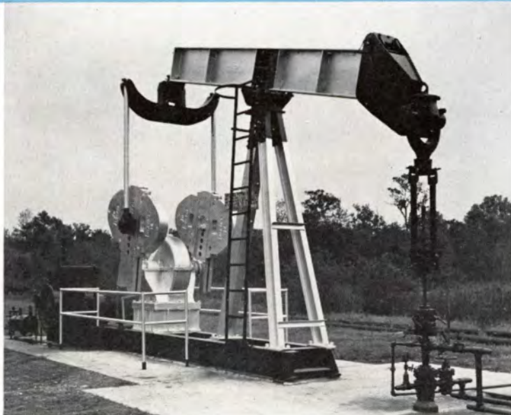
LUFKIN TC-2A-36 UNIT, driven by Lufkin Cooper-Bessemer Engine, Amerada Petroleum Corp., Bunkie, Louisiana.
