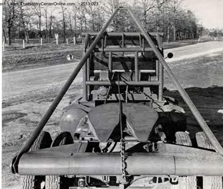
This truck is completely outfitted for oil field work by Lufkin's Trailer Division. Model 15 Winch is used for float trailer and gin pole service.
