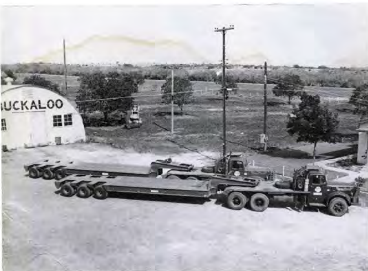
THESE three-axle low-boys can haul 125,000 pounds easily. Lower gravity loads mean safer handling
