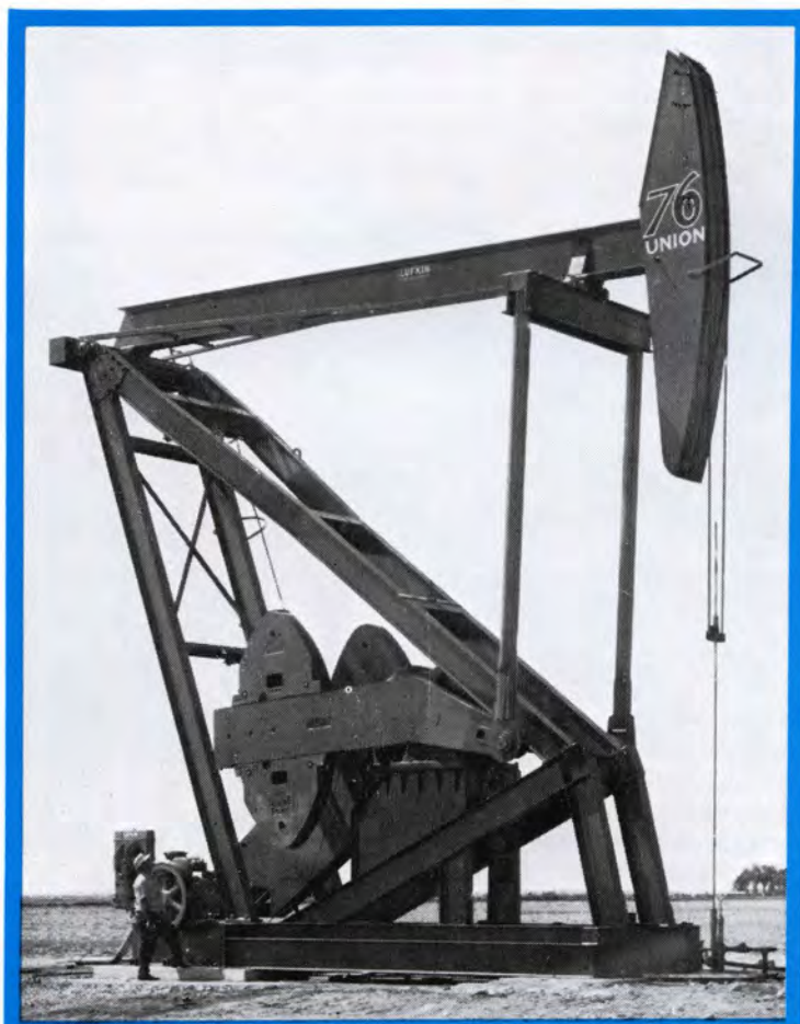
LUFKIN M-640D-305-192 UNIT, DRIVEN BY A LUFKIN H795 ENGINE UNION OIL COMPANY OF CALIFORNIA, FARNSWORTH, TEXAS
