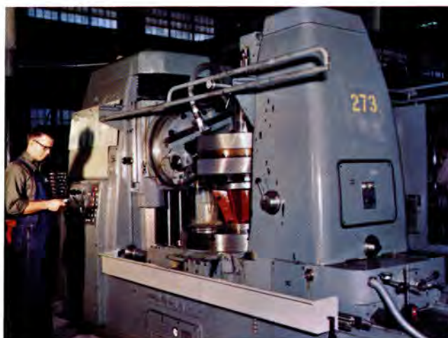
THIS Pfauter is one of several high precision gear hobbers.
