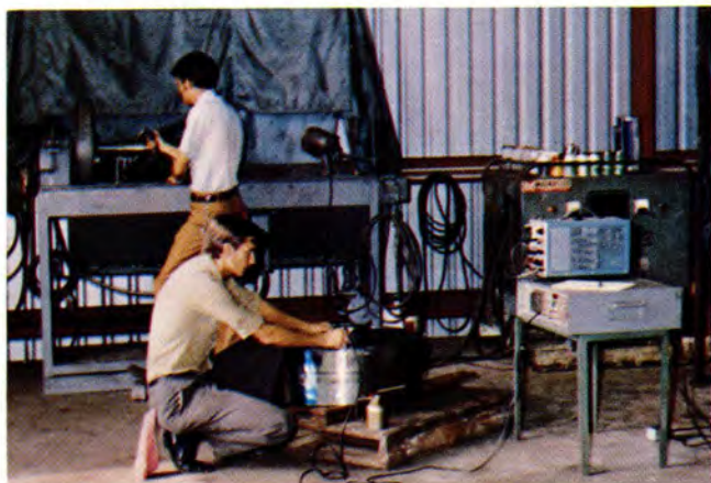
MATERIAL quality is assured by using ultrasonic and Mag-naglo inspection equipment. All forgings are certified before final machining
