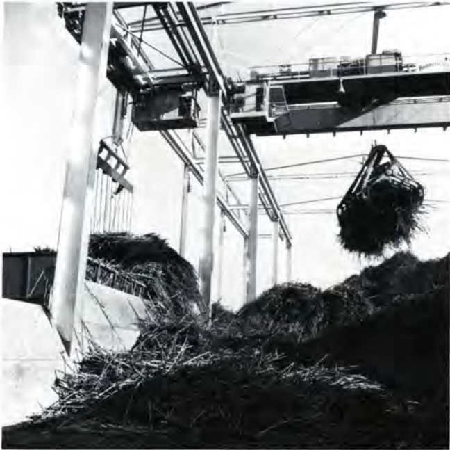
Cane unloaded from wagons during daytime hours keep the mill fed at rate of 250 tons per hour
