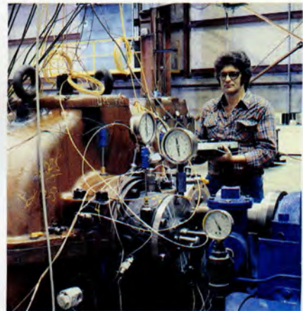
Technician Clarence Miller performs a load test on a LUFKIN N1604 Gear Increaser, a unit designed to transmit 1,750 horsepower from an electric motor to 1,750 RPM to a centrifugal compressor at 8,986 RPM.
