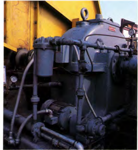
A LUFKIN NM1800C Gear Reducer transmits 850 HP from a steam turbine at 4,554 to a cane knife at 602 RPM in a sugar mill.
