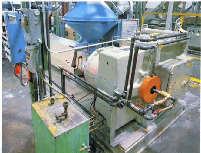
In a Georgia chemical plant, a LUFKIN D315-921C Extruder Drive operates at 1,750 RPM input, driving an extruder screw at 74 RPM.
