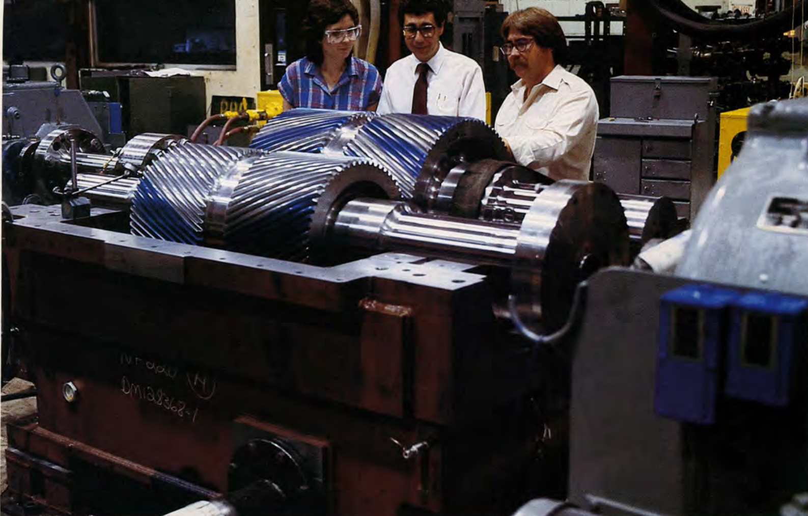
(l-r) Lisa Ford, design engineer, George Adda, LUFKIN sales representative, Pittsburgh, and Rick Masters, design engineer, check gear tooth contact on the NF2207C prior to testing.
