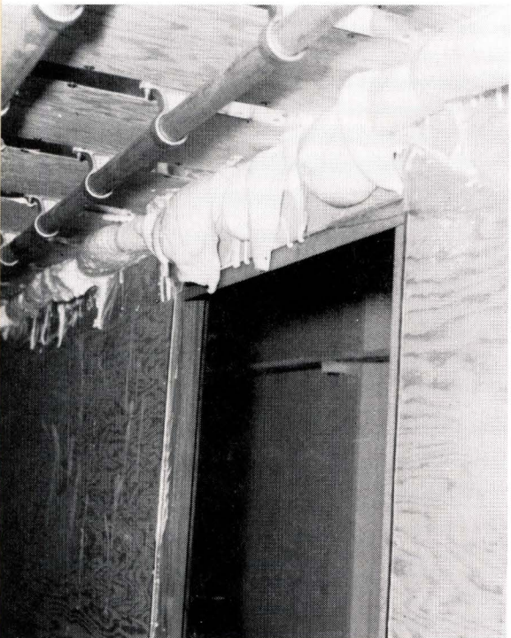
THIS is a meat rail trailer. The white bulges are foam which has spilled over from the sides. In this instance, the sides were foamed up to the last three inches, which was later covered with some type of flashing material. Then the roof was foamed from outside the trailer in the same manner as foaming the floor
