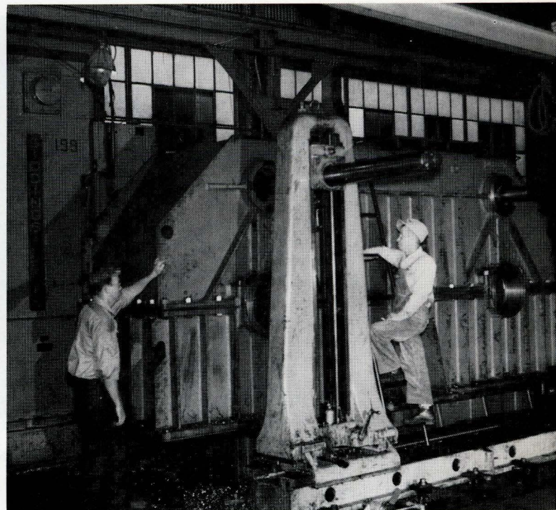
AFTER all sections were drilled, they were bolted together and put on the horizontal boring mill for finishing of the bores for shafts and pinions. Employees shown here are JIMMY HAWTHORN, left, and KERNS BAILEY.
