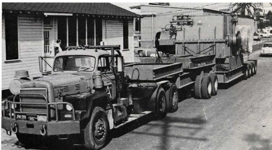
16. THIS UNIQUE 300-ton low-boy trailer was required to transfer the gear unit to Pascagoula, Mississippi, for assemblage with the ship's engine. The trailer's 56 huge tires rolled the gear down Kiln Street where a crowd of office and shop employees gathered for one last look.
