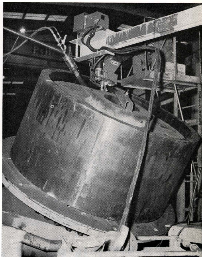
3. MEANWHILE, the procedure is underway of welding the gear "blank," the name for a gear without the teeth cut. Here the spherical "hub" has been welded to the "webs," round discs which, when welded inside the gear blank's outer rim, will provide internal stress for strength. Pictured is Ronnie Hunt, Welding Shop, first shift.
