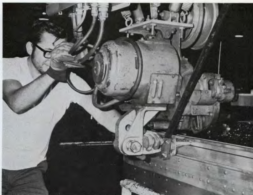
9. IN THIS VIEW atop the platform shown in the previous picture, Billy Joe White is stitching the roof to the sides. The metal stitching, which is similar to a series of common office staples although many times stronger, has one-inch centers for maximum holding power. Only about a minute and a half are required to stitch both sides of a 40-foot van. After the stitching, the back edge of the roofing is cut from the coil and neatly trimmed later when the back doors are affixed. With three sides and a roof, the section now is referred to as a "box."
