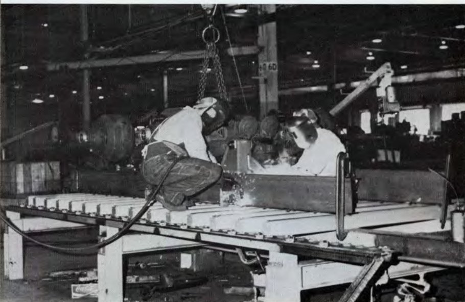
11. NEXT STEP is welding together the parts of the chassis, known at this point as the sub-assembly. Here Edward Clifton, left, and Brown Hayes finish a running gear.
