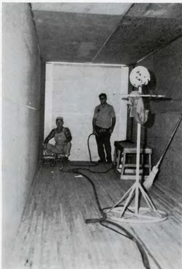
13. NOW the two assemblies are joined as the box is set on the chassis, which has been levelled prior to this. Flanges are fitted around the wood flooring on the chassis. Left to right are Billy Joe White, Curtis Grimes, Fred Nash and L. M. Hodges.
