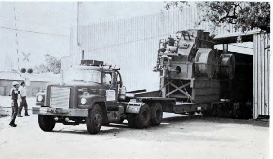
BELOW: A winch was used to pull the truck with its 150,000-pound load from the gear building, which has a wide door to accommodate LUFKIN's largest units
