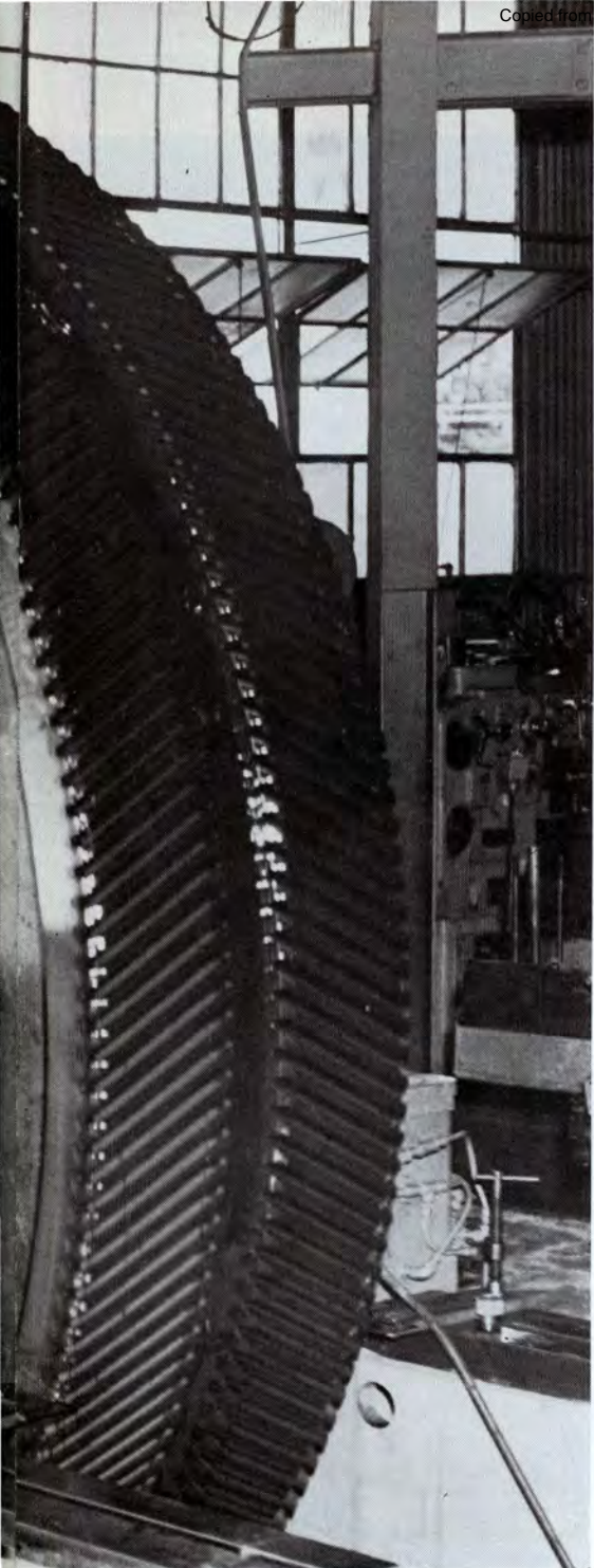
BILL POE, Commercial Gears, first shift, installed an oil line on the unit as it was nearing completion. The marine gear has a rating of 12,000 horsepower
