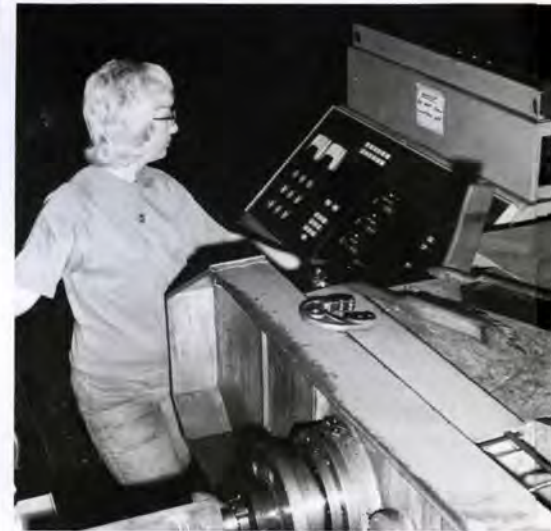
Artha Boles, 3rd shift, operates this numerically controlled 311 lathe which machines crank pins and reducer shafts
