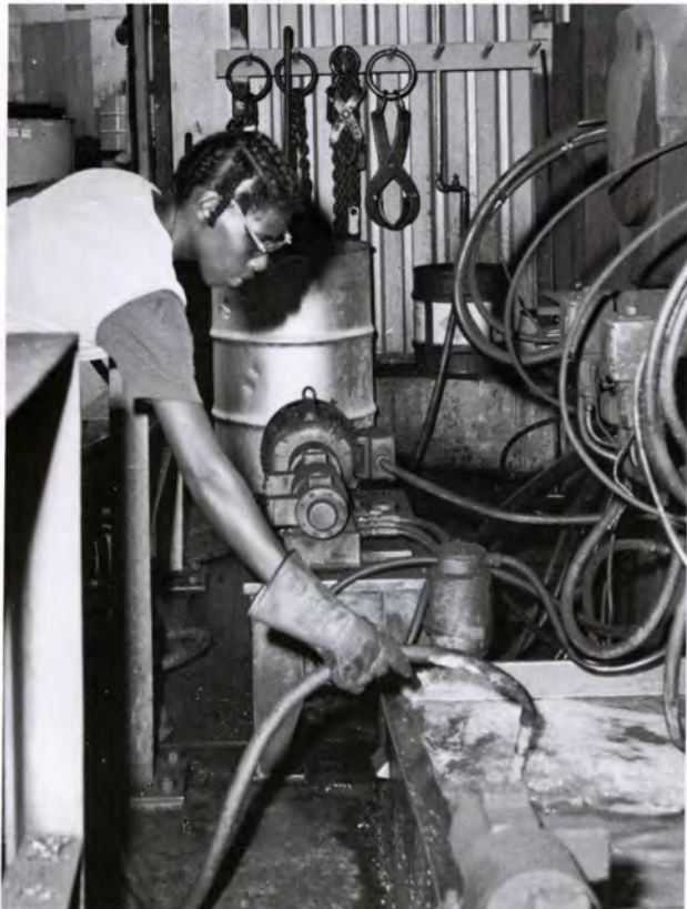
"Watering the machines" or running water on the cutting tool, as Mary Etta Patton, Lathe Shop, 2nd shift, does, keeps this lathe from overheating after prolonged use
