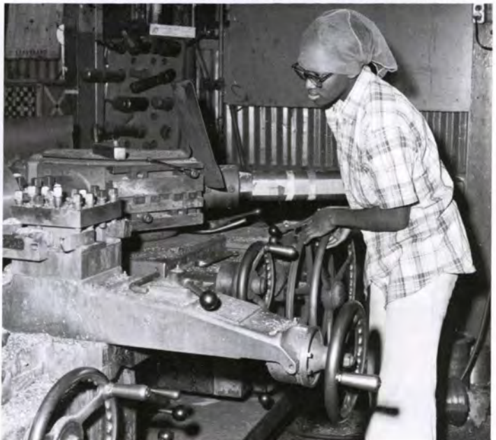
As a machine operator trainee, Sadie Jones is learning to run this Turret lathe which bores and turns parts to precision dimensions
