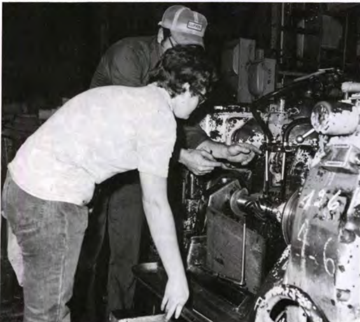
Trainee, Linda McDiffett receives instruction from Robert Barbe, 1st shift, on how gear teeth should look after being cut properly
