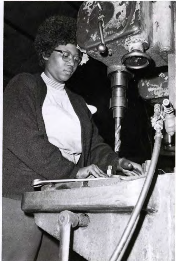
"Watering the machines" or running water on the cutting tool, as Mary Etta Patton, Lathe Shop, 2nd shift, does, keeps this lathe from overheating after prolonged use
