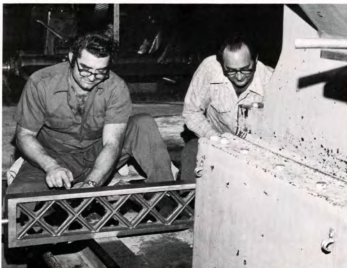
Bill Sides, left, and Buddy Atkinson are handscraping the bedway of a 5B generator purchased in 1937 in order to make alignments and bearings fit
