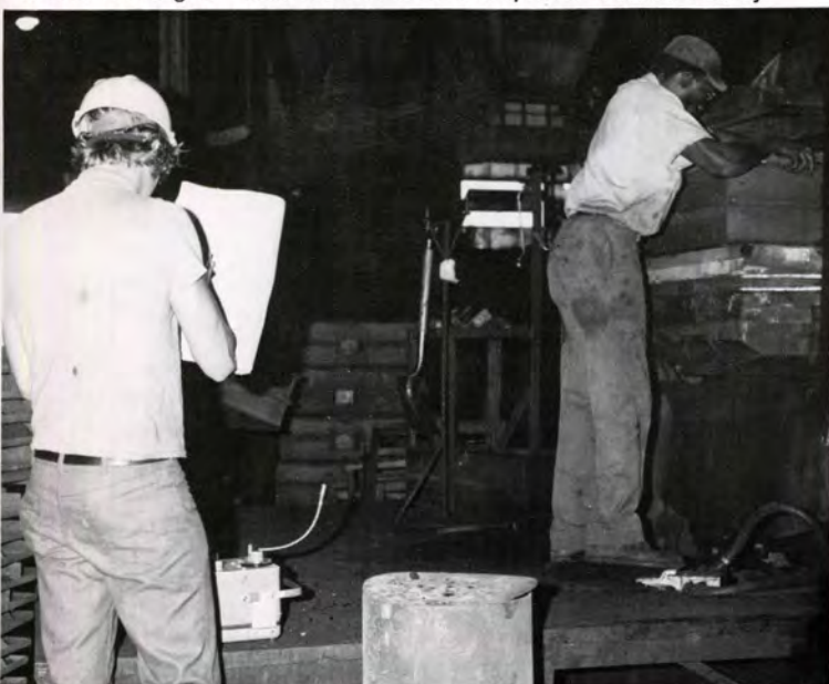
As Jim Singletary, foundry side bay, right, rams a mold, Betz engineer records reading on noise monitor with microphone located nearby
