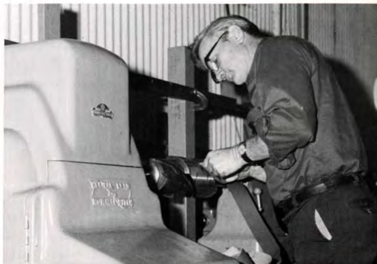
Jim Peavy is handscraping guides to correct lead. The guides place the helix angle on a part
