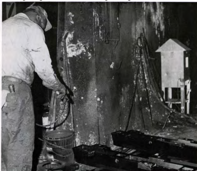
R. D. Forney, assembly and shipping, spray paints pumping unit bases. As he paints, the shiny box structure in the background in the paint booth is measuring the fumes by drawing a high volume of air through a large filter
