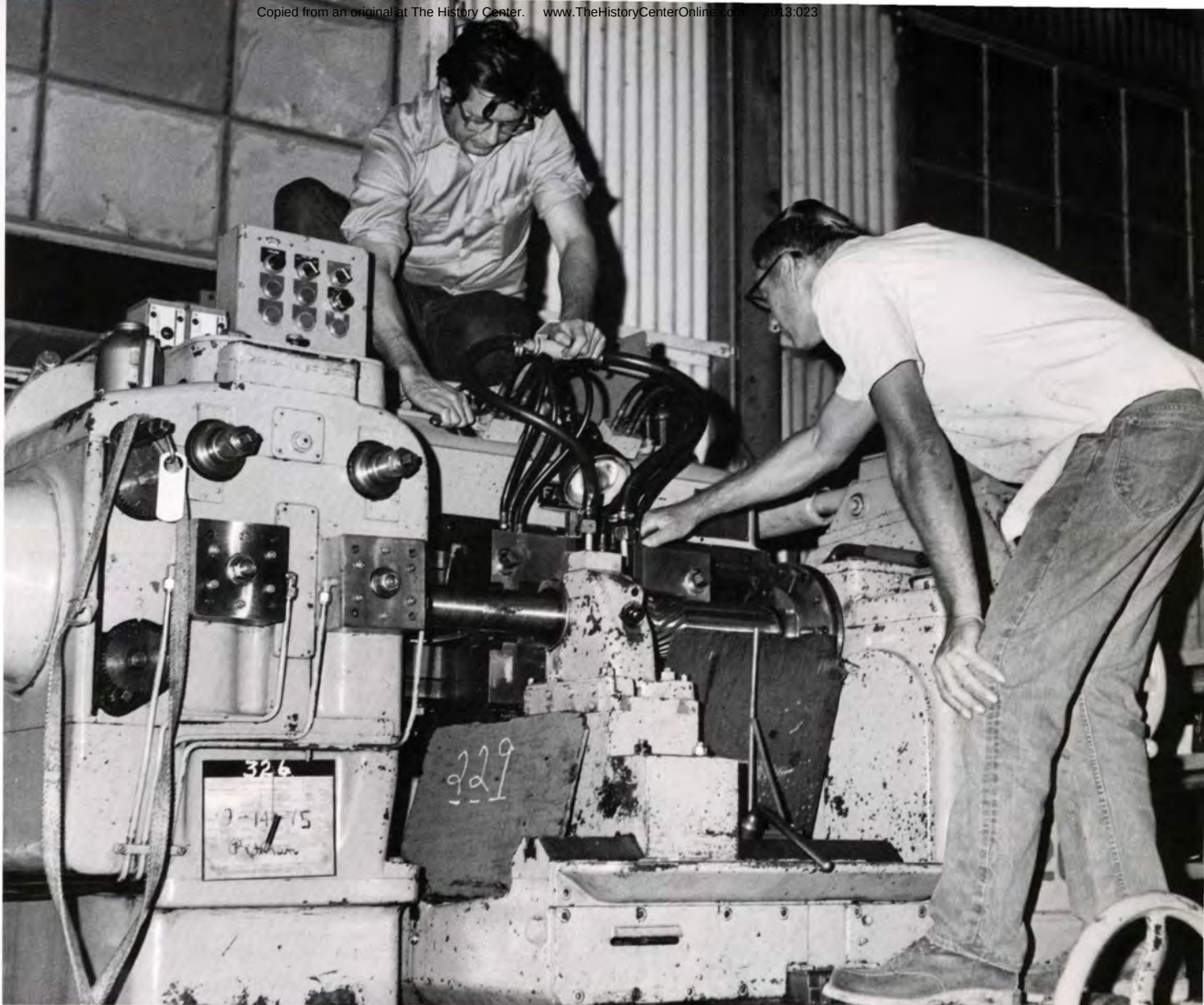
Don Anderson, top, and Fred Peterson are replacing a hydraulic hose on a cutter head. LUFKIN employees designed and built the cutter heads which can be used only on hydraulic machines. The heads were designed six inches shorter to improve the visibility for the machine operator.
