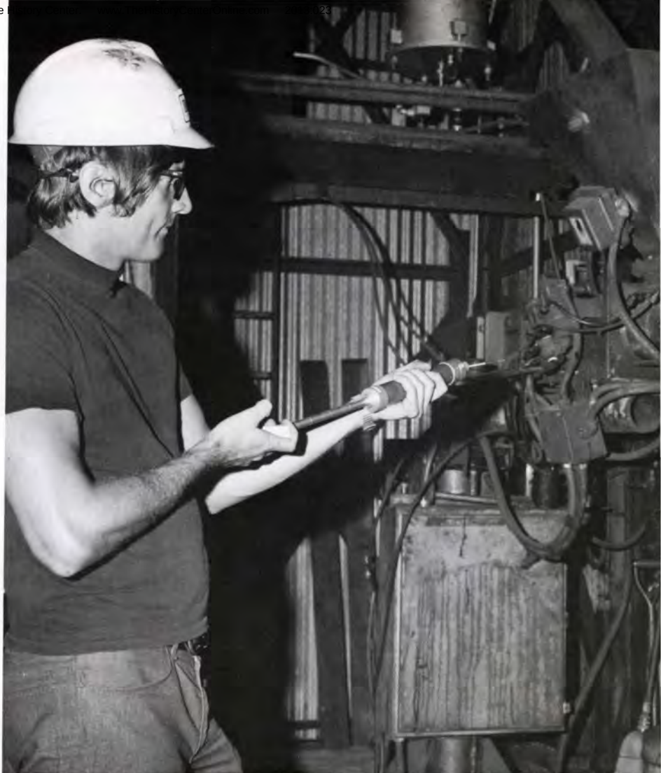
Using a hand pump with a glass tube attached, Magnus Leopold, Betz engineer, takes an air sample around the no-bake mixer in the foundry core room
