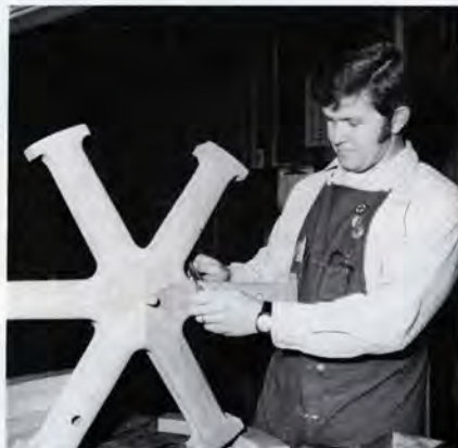
Larry Vann puts finishing touches on pattern for a spoke of a sheave for a pumping unit
