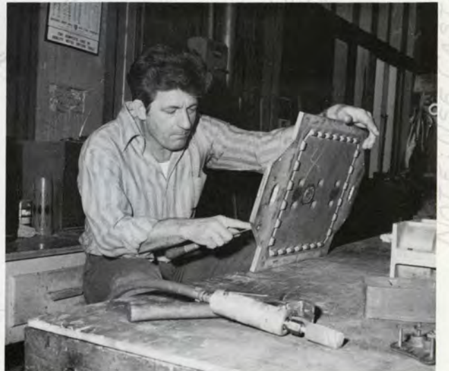
Vernon Nixon files and cleans a master pattern
