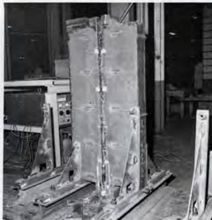
A new Hobart porta-slag welding machine joins two slabs into one solid piece of steel. The savings on one job amounted to $122
