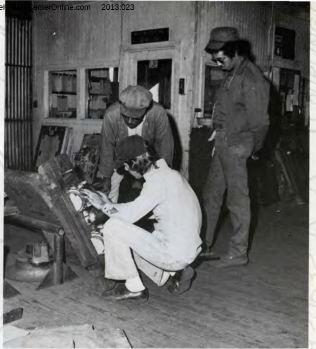
Gary Selmon, kneeling, works out a minor repair on a pattern while pattern hustlers Willie Mitchell and Elton Menefee, right, wait to take the pattern back to the foundry
