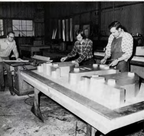
Jerry Palmore, left, cuts wood to size while Ken Ramsey, center, and Billy McClendon check measurements of a new multiple pattern for weights
