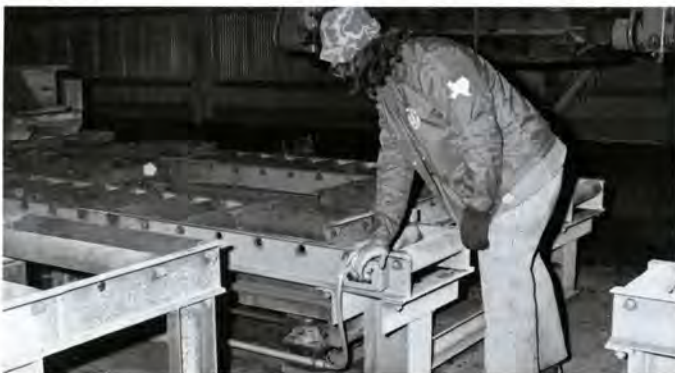
Four screw jacks powered by \frac{3}{4} h.p. electric motor lifts up the pattern even to the pattern return conveyor. Georgia Bryan, 1st shift, is lowering the lift station
