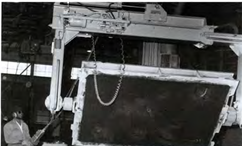
Charles Holman operates the new rollover machine that has a capacity of 6500 pounds. It is the largest rollover machine Donovan manufactures
