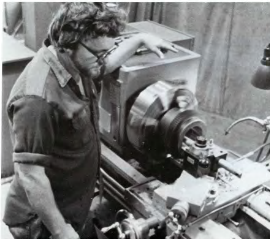
James Cates, jig shop, 1st shift, said the new LeBlond lathe makes his job a lot easier because of the trav-a-dial that gives a longitudinal measurement
