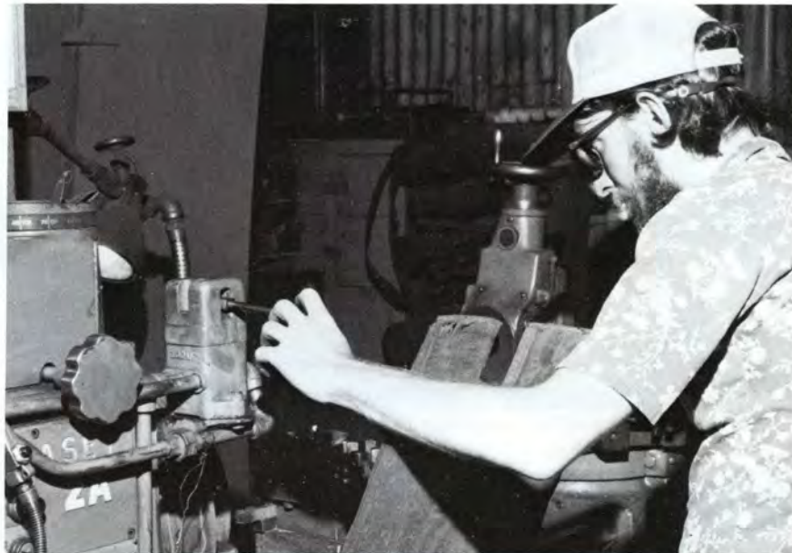
Joe Ericson, lathe shop, 3rd shift, runs the Warner Swasey No. 2A turret lathe recently installed in the lathe shop
