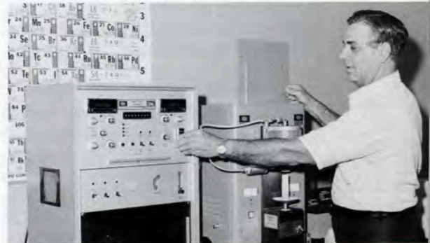
Frank Martin, chief metallurgist, operates a LECO machine that analyzes small quantities of carbon and sulphur
