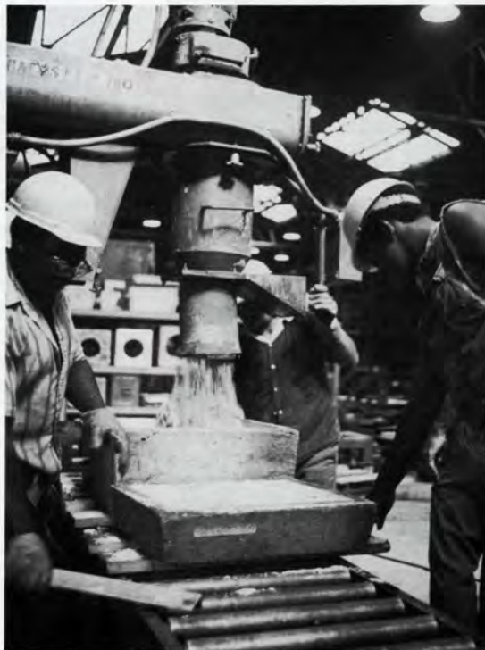
Roger Herst (Left) and Yule Brown, both core room, 2nd shift, fill cope and drag using pep set process. (Right) Pedro Rodrigues is pasting drag so cope can be placed.
