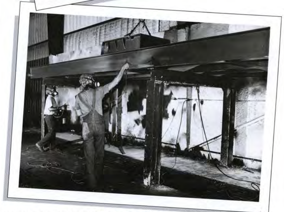
Top, (l-r) Robert Elliott and M. H. (Red) Patrick prepare to move a group of ladders from the shot blast area to the paint booth. The department shot blasts more than two million pounds of metal each week, averaging 345,000 pounds of metal each 24-hour period. Below, one safety feature of the new paint booth is a permanent holding rack. The rack is used, in addition to overhead cranes, to support larger parts while they are painted. In case of a power failure, there is no danger of a part dropping from an overhead crane. Pictured (l-r) are Billy Hoosier and Robert Elliott
