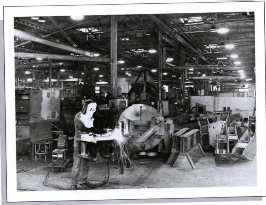
Top, after a profile change by a manufacturer, the 88-pound beam used in pumping unit bases could no longer be purchased. Company maintenance and electrical crews designed this welding machine for fabricating the necessary beam. It is housed in Bay 9. Below, a new lighting system of high pressure sodium lights provides twice the illumination of the old mercury vapor light system for the same amount of energy consumption.
