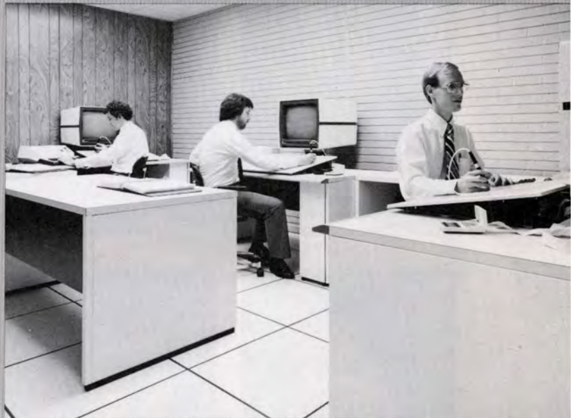
The computer graphics operation is located in a wing of the engineering department that is built 12 inches off the ground. Underneath the floor is a heating and cooling system which maintains a constant temperature of 68 to 70 degrees in the room. If the computer becomes too warm, it will automatically turn itself off. Pictured are computer graphics designers (l-r) Ted Slemmons, Jerry Taylor and John Milton.
