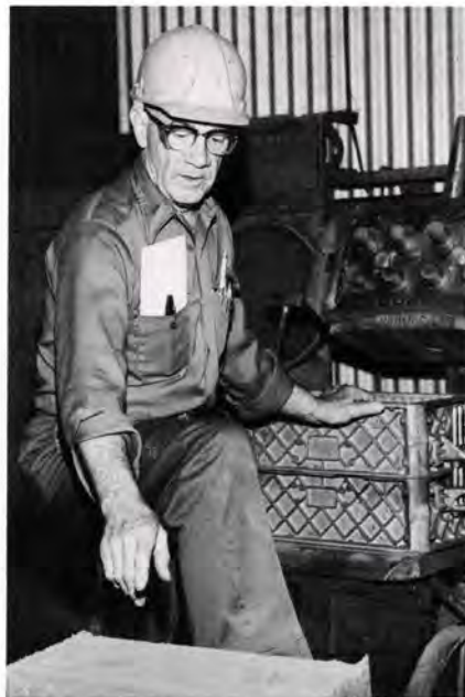
Houston Davidson demonstrates one of the first molding machines purchased by LUFKIN. The machine is used in the bronze foundry to make molds for small aluminum castings.
