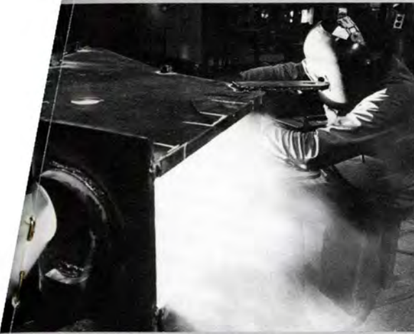
(4) The welding & structural shop fabricates steel into parts that later will be assembled with casted, machined parts from the foundry and machine shop. Pumping unit parts such as the horsehead, the walking beam, the sub-base, the base and samson posts are structured in this area. (5) In the pumping unit gear box assembly area, the gear reducer is assembled from machined parts. Here, Manuel Basham tests gears for any burrs, before they are joined to other parts. In the background, Lunell Curl puts bolts in the gear. The sub-assembly area, housed in the same building, assembles smaller items. (6) The Trailer Division began assisting in the production of 114D pumping units in 1979. Last year, they structured and assembled 1,430 units. Curtis Grimes installs brake handles on a unit.
