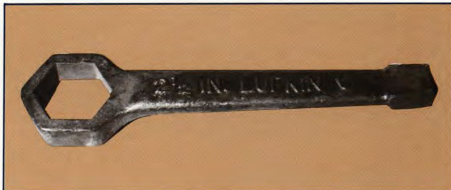
Below, a LUFKIN pumping unit wrench is on display in the Pistol Hill Gas Station exhibit in Boomtown. The wrench was used for removing wrist pins. Left, visitors to Boomtown can stop and watch a machinist of the 1930s at work in the Wright City Machine Shop. The Museum is located on the Kilgore College campus facing U. S. 259. It is open from 9-4 Tuesday through Saturday and 2-5 Sunday.
