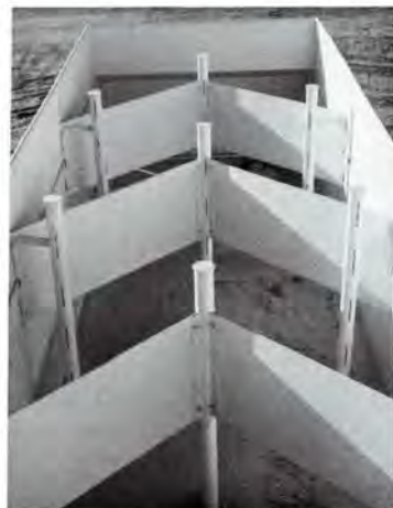
Left, Extra height was added to the trailers to keep water from splashing over the sides of the dumps. Middle, Pictured in an inside view of the trailers after the wave breakers were installed. The breakers absorb movement of the load during transporting. Right, The anchovies are unloaded to the catch hole at the fishmeal processing plant. Note the net covering the top, of the trailer which is designed to protect against sea gulls.
