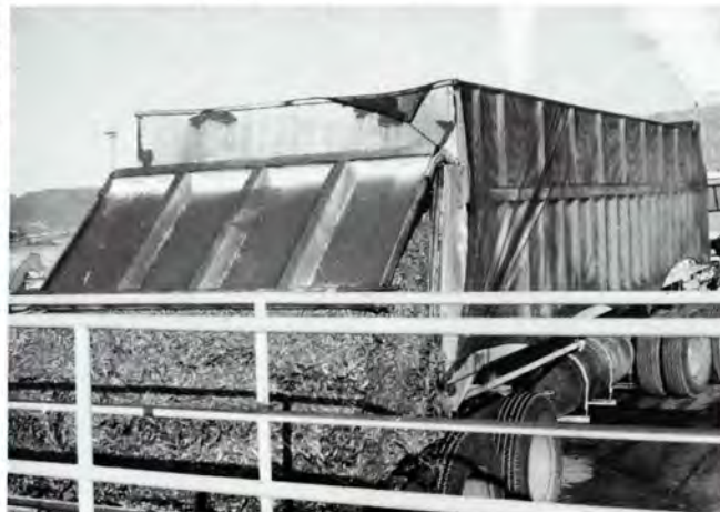
Left, Extra height was added to the trailers to keep water from splashing over the sides of the dumps. Middle, Pictured in an inside view of the trailers after the wave breakers were installed. The breakers absorb movement of the load during transporting. Right, The anchovies are unloaded to the catch hole at the fishmeal processing plant. Note the net covering the top, of the trailer which is designed to protect against sea gulls.
