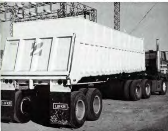
Left, Extra height was added to the trailers to keep water from splashing over the sides of the dumps. Middle, Pictured in an inside view of the trailers after the wave breakers were installed. The breakers absorb movement of the load during transporting. Right, The anchovies are unloaded to the catch hole at the fishmeal processing plant. Note the net covering the top, of the trailer which is designed to protect against sea gulls.
