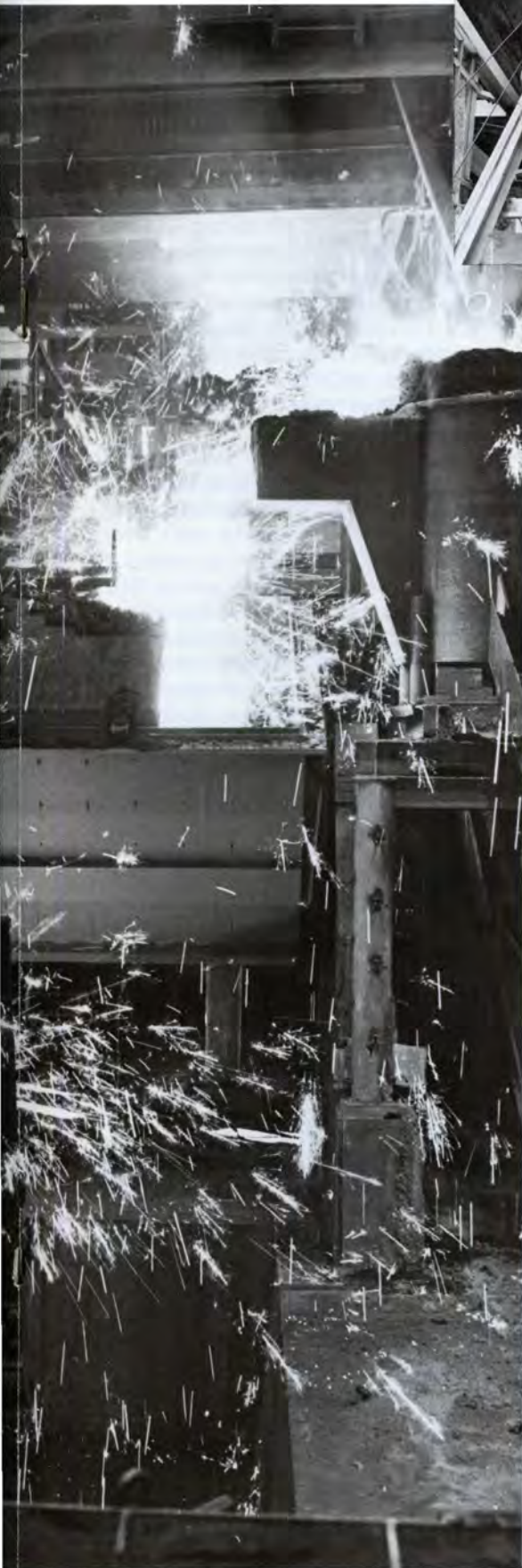
The new melting system began operation in late September. Here, foundry employees observe the automated system of charging for the first time. As raw materials are needed by the cupola, they are moved by conveyor to a holding bucket and mixed with structural steel or scrap iron. The mixture is moved into the cupola by an oscillating feeder.
