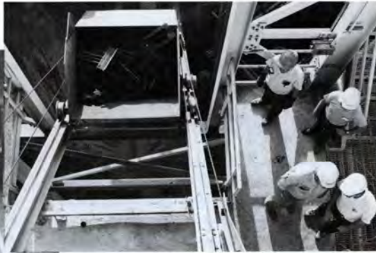
The new melting system began operation in late September. Here, foundry employees observe the automated system of charging for the first time. As raw materials are needed by the cupola, they are moved by conveyor to a holding bucket and mixed with structural steel or scrap iron. The mixture is moved into the cupola by an oscillating feeder.
