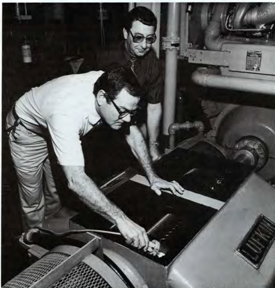
Bishop and West India Shipping Company marine superintendent C.C. Carter inspect the gear wear pattern of a LUFKIN marine unit installed on the ship, The Inagua Beach. Bishop periodically inspects LUFKIN units that are operating in his territory. This installation was sold in 1969.
