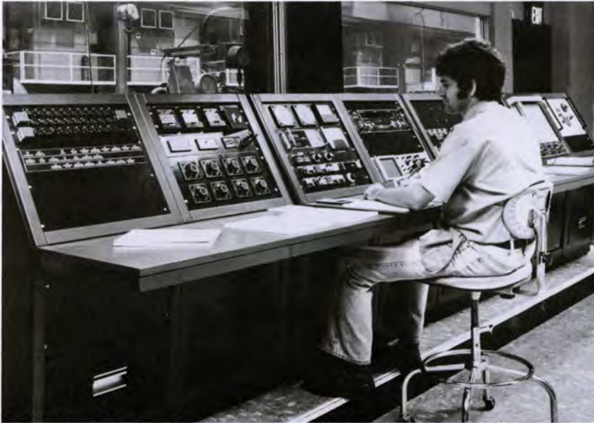
(Opposite page) The new gear testing facility features testing areas for both high-speed and low-speed gearing. Pictured are (l-r) Jimmy Foster, quality assurance technician, and Charles (Doc) Grimes, inspector. (Above left) Technician Clarence Miller monitors a test in the instrumentation room. The test panel is designed to provide data display and recording, control of test parameters and instrumentation for diagnostics of gear quality problems. (Above right) The new test stand features two levels of offices. Offices for Leonard Avery, manager of the gear test and service department, and Betty Havard, test coordinator, are located on the first floor.
