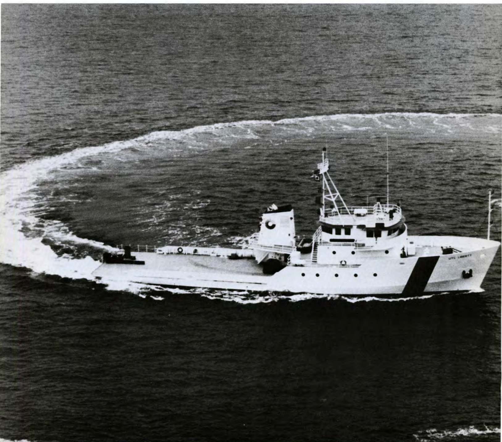
Soon after the Columbia has disappeared into space, the UTC Liberty and her sister ship, the UTC Freedom, are at work reclaiming the rocket boosters from waters off the east coast of Florida. On board are 24 crewmen and retrieval specialists. (Photo courtesy of United Space Boosters)
