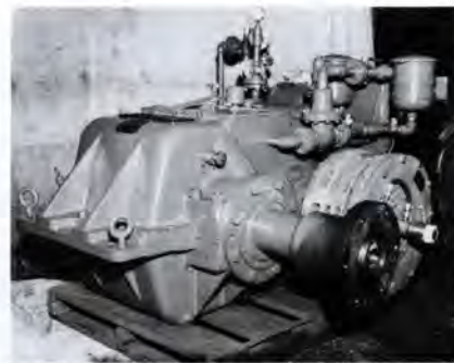
For open ocean travel, the vessels are powered by twin diesel engines and are equipped with two LUFKIN HSQ2120 marine reduction gears. The LUFKIN HSQ1616 marine gear (pictured) is similar to the HSQ2120 marine gears used in the ships.
