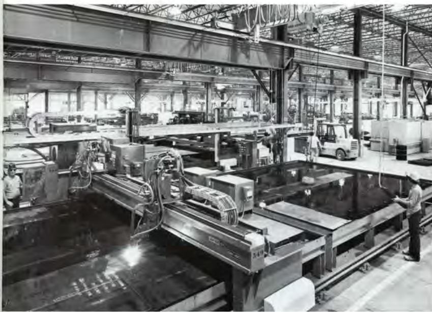
(Top, Left) In the foreground is a new plasma arc shape-burning machine. Behind the plasma arc is the torch cutting machine, which is equipped with eight oxy-fuel torches. Both machines are CNC controlled and used for burning shapes used in pumping units. (Bottom, Left) The roll over positioner is being used to weld out a base. The positioner rotates the base to any position for welding without the use of overhead cranes. (Below, Top) On February 26, the first domestic pumping unit was loaded for shipment from one of the eight loading docks in the shipping department. (Below, Bottom) Final assembly and shipping facilities occupy 67,500 square feet. This photo shows half of the assembly building, which is presently being used for production. One of the three 15-ton semi-gantry cranes is shown. The two paint booths are behind the crane.
