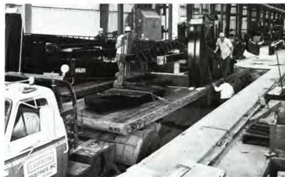
(Top, Left) In the foreground is a new plasma arc shape-burning machine. Behind the plasma arc is the torch cutting machine, which is equipped with eight oxy-fuel torches. Both machines are CNC controlled and used for burning shapes used in pumping units. (Bottom, Left) The roll over positioner is being used to weld out a base. The positioner rotates the base to any position for welding without the use of overhead cranes. (Below, Top) On February 26, the first domestic pumping unit was loaded for shipment from one of the eight loading docks in the shipping department. (Below, Bottom) Final assembly and shipping facilities occupy 67,500 square feet. This photo shows half of the assembly building, which is presently being used for production. One of the three 15-ton semi-gantry cranes is shown. The two paint booths are behind the crane.
