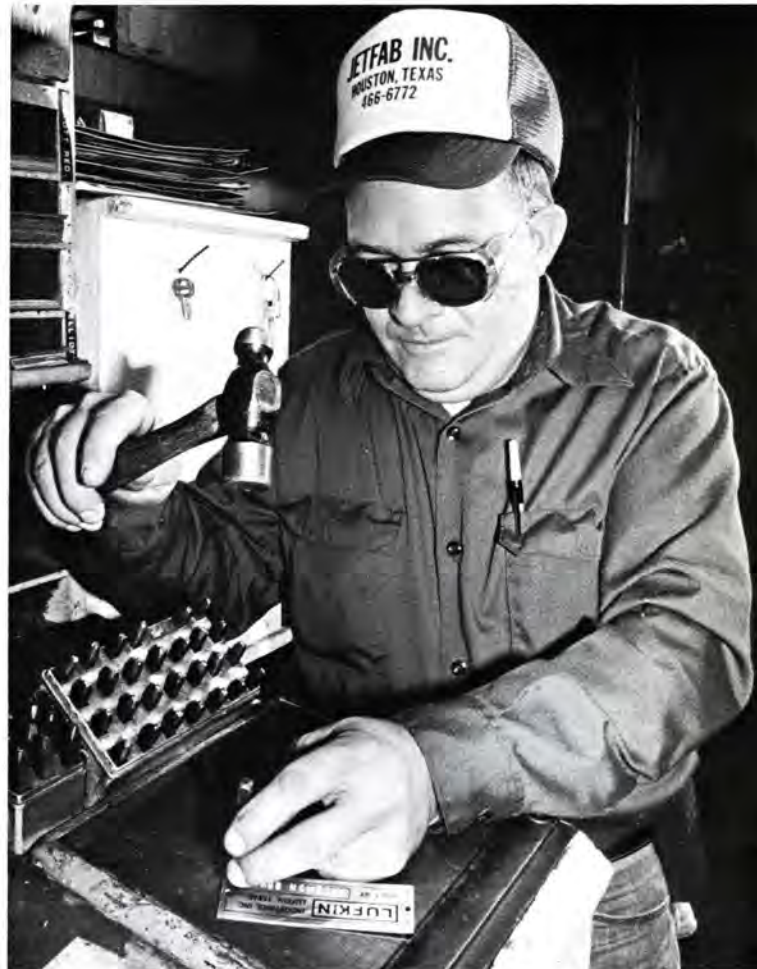
Sam Turner stamps the names of assemblers and pipefitters on identification tags. Quality control personnel tag the units after final inspection.
