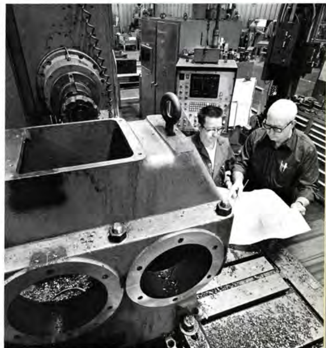
Left, quality control employee Ronnie McMullen updates the "quality parts only" board that hangs in the industrial gear machining area. The number of days of manufacture of only quality parts are posted for each shift. Right, Ed Pillows and Hubert Lankford double check machining specifications for a gear box. If a part has to be returned to a work station for further machining, it is considered a rework piece and non-quality part.
