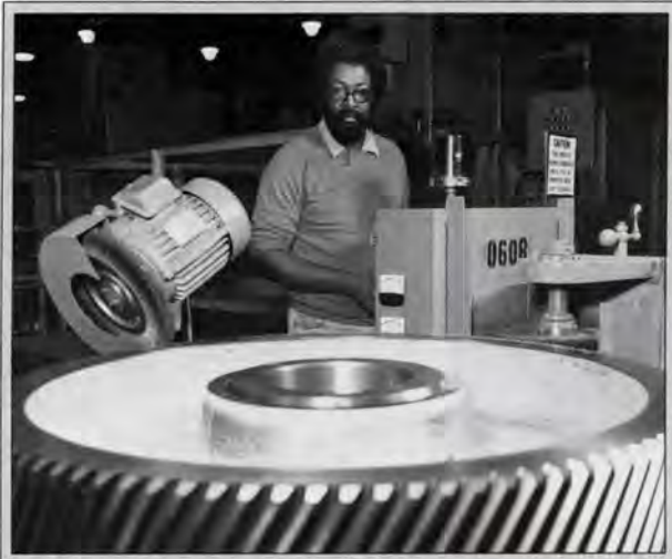
Walter Levine, machine shop assembler, operates a machine that removes metal burrs from between teeth on a Mark II slow-speed gear. Photo by Viron Barbay
