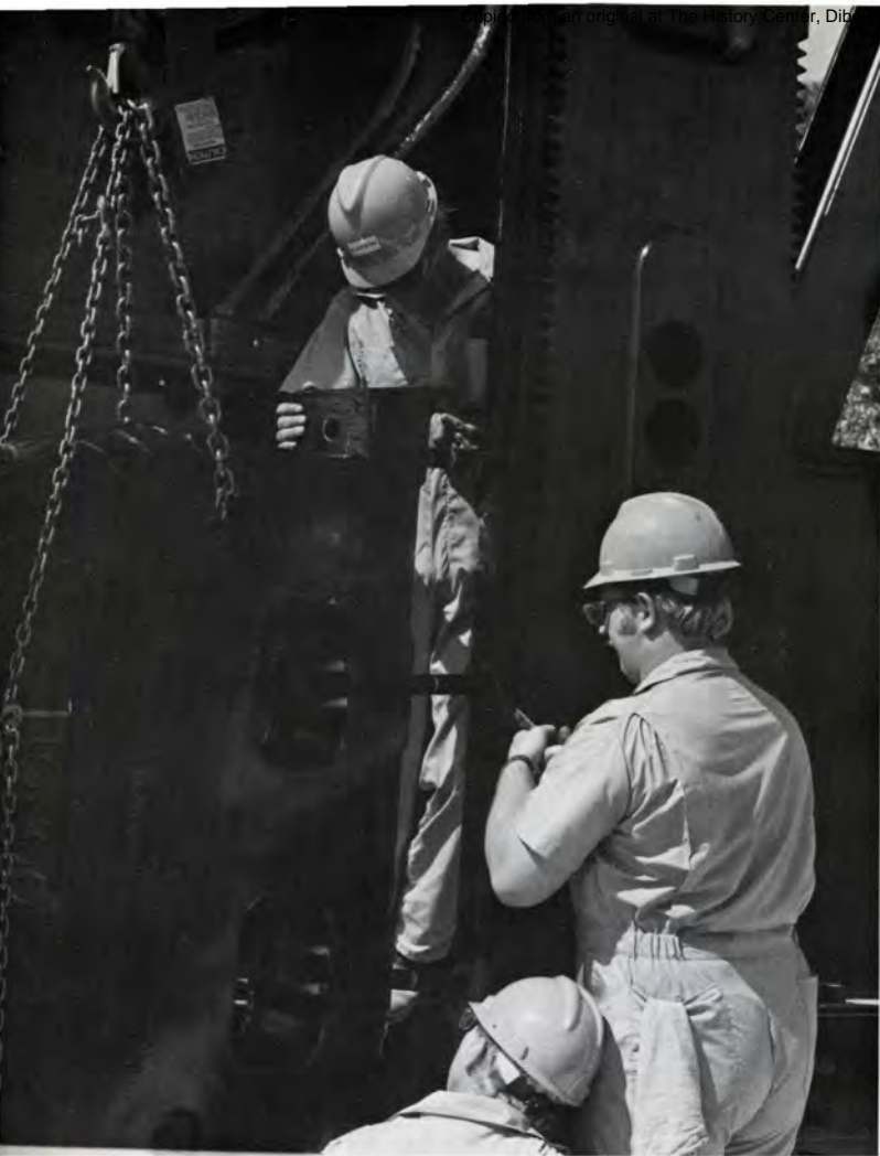
Left: W.Z. Hutson (top), John Bridges (middle), and T.J. Reynolds (bottom), guide a counterweight into position for mounting on one of the C1280 cranks.
