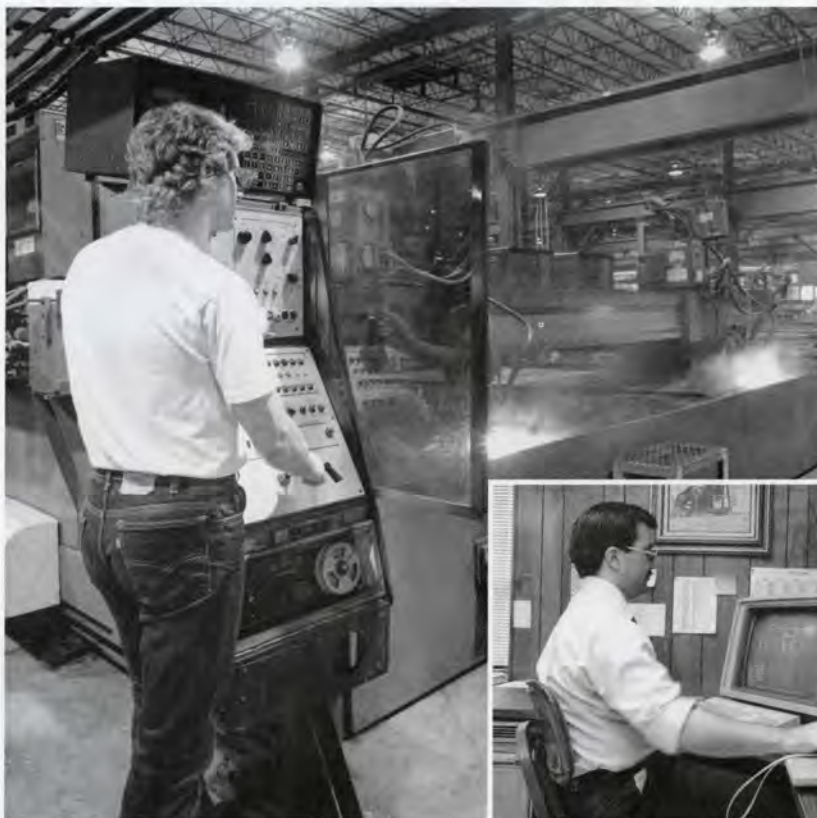
Rick Huckabee, Burner, watches the cutting operation of a horsehead that was programmed through the computer located above the controls. The tape reel, located at the bottom of the control panel, has been eliminated. Inset: David Meaux, NC Operator, designs a tool path for machine operations.
